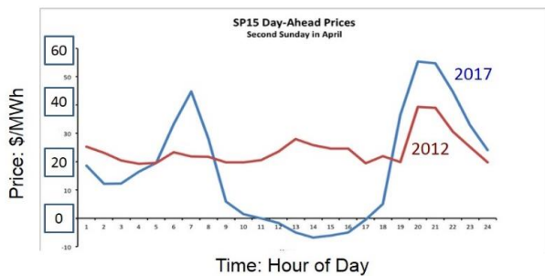
Fig. 6. Changes in wholesale electricity prices in California on a spring day due to the addition of solar PV
