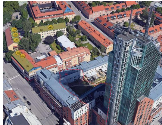
Fig. 7. The above image, as part of Vasteras city center, shows (a) the shadow cast by the surrounding tall building, (b) the roof obstacles, (c) the different building slopes, and (d) the different building orientations.
