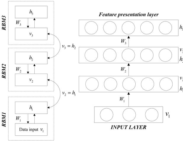
Fig. 2. The structure of Deep belief network.
