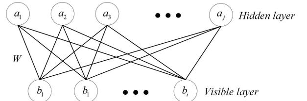
Fig. 1. The structure of Restricted Boltzmann Machine.
