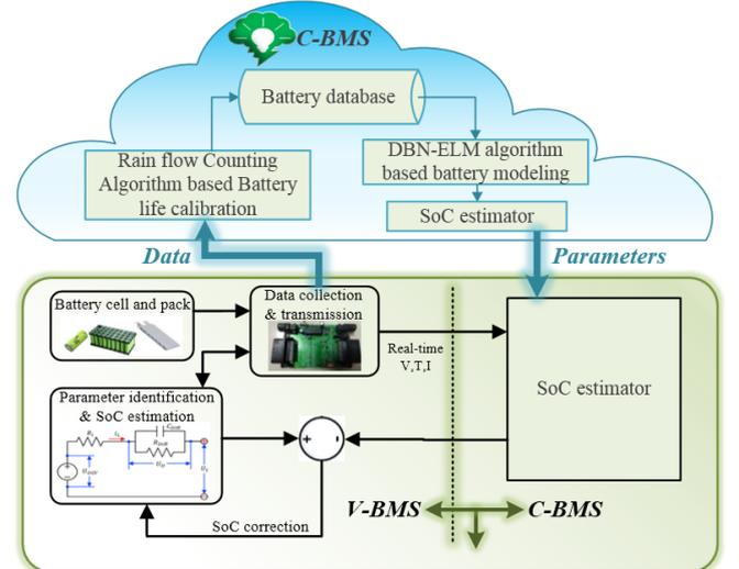
Fig. 3. The conjunction working mode between C-BMS and V-BMS.
