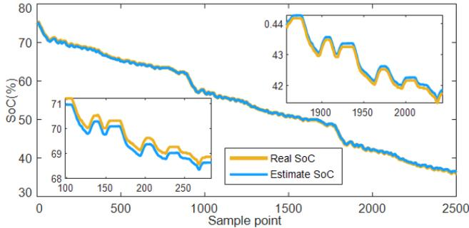
Fig. 10. The accuracy SoC estimation based on the proposed conjunction working mode between C-BMS and V-BMS.
