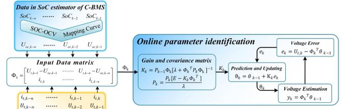
Fig. 5. Battery parameter identification method based on the conjunction working mode between C-BMS and V-BMS.
