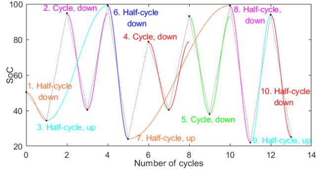
Fig. 8. The result of rain-flow cycle counting algorithm based battery degradation quantification method.
