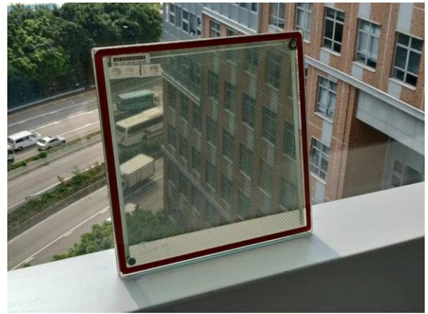
Fig. 3. The front view of the vacuum PV glazing
