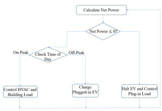
Fig. 3. Admin Microgrid Proposed Strategy: While Trolley is unavailable
