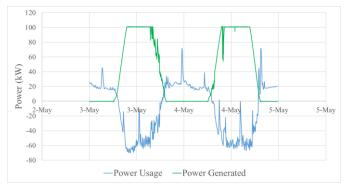
Fig. 5. The net zero administration building: PV generation and usage
