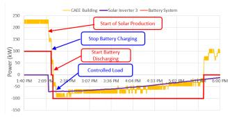
Fig. 7. CAEE Building demand deduction and net power fed back to the grid on RPU's voluntary load shedding request
