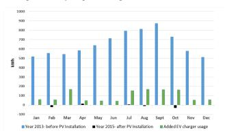
Fig. 6. Net zero demonstration: CE-CERT Administration Building daily average electricity usage from grid before and after PV installation
