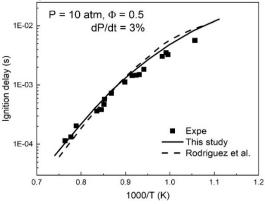
Fig. 3 Ignition delay comparison between experiment [14], model in this study and model by Rodriguez et .al for MOD9D/air mixture: P = 10 atm,  $\Phi$  = 0.5.
