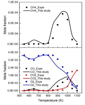
Fig. 6 Comparison of species mole fraction in PSR between model in study and experiment.
