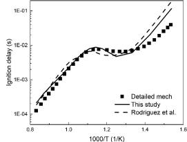
Fig. 2 Ignition delay comparison for MOD9D/air mixture at 13.5 bar and stoichiometric condition.
