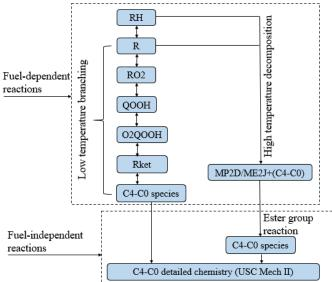
Fig. 1 Simplified schematic oxidation pathway for heavy unsaturated methyl esters.
