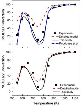
Fig. 5 Comparison of conversion rate of MOD9D and NC10H22 in PSR between experiment [16], the detailed model, model in this study and Rodriguez's model for n-decane/MOD9D fuel mixture at 1 atm, 1.5s, 0.2% fuel (0.26 MOD9D/0.74 n-decane) at  $\Phi$  = 1.0 with He diluent.
