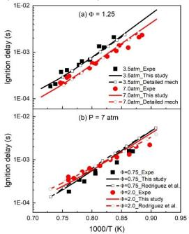
Fig. 4 Ignition delay comparison between experiment [15], model in this study and the detailed mechanism for MOD9D, (a)  $\Phi = 1.25$ ; (b) P = 7 atm, in 4% oxygen/argon mixtures.
