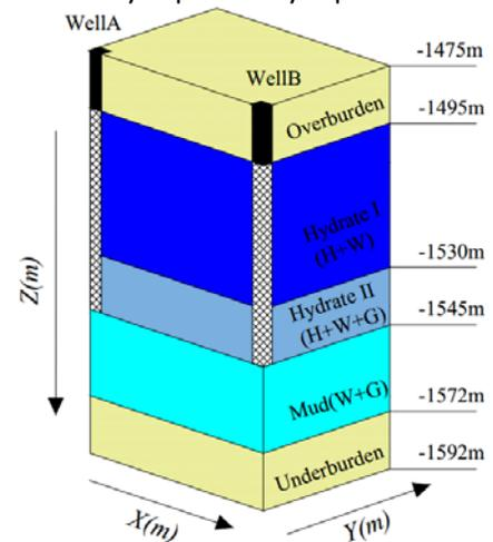
Fig 1. The schematic diagram of physical model at W17 site between two vertical wells in multi-vertical well patterns
