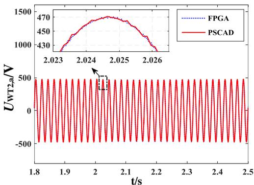
Fig 7 Phase-A voltage of PMSG unit 2
