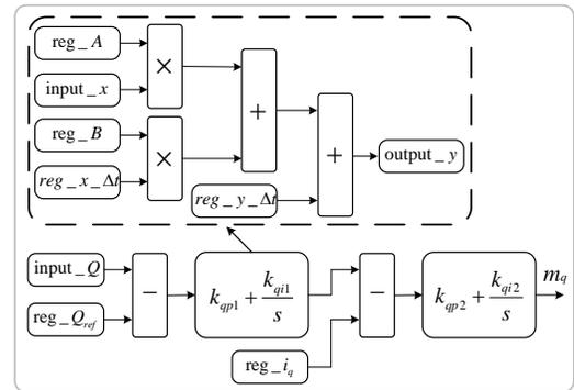
Fig 2 Hardware design of the q-axis model based on FPGA
