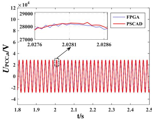
Fig 5 Phase-A voltage of PCC
