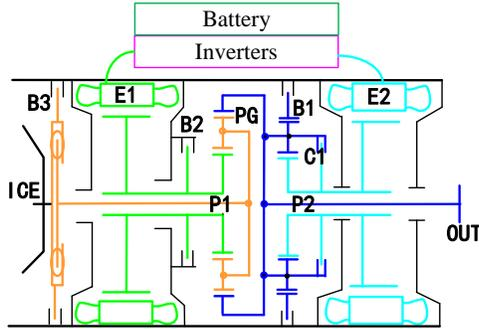
Fig 1 Configuration of dual-planetary gear
