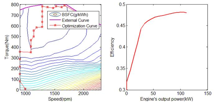
Fig 2 Relation between engine's efficiency and output power
