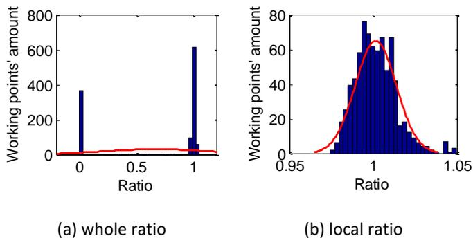
Fig 8 Ratio of ICE's output power to total driving power
