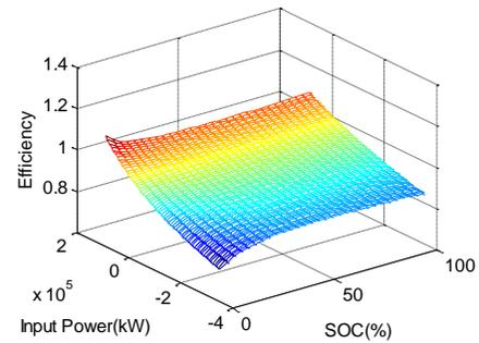
Fig 3 Battery's efficiency
