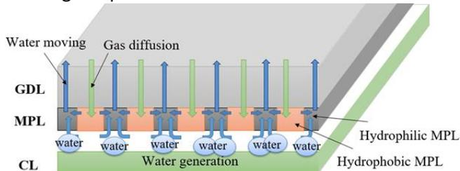
**Fig. 1.** Structure and function of the MPL exhibiting planar wettability.
