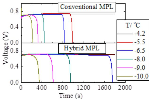
**Fig. 2.** Voltage changes of PEFCs using conventional and hybrid MPLs when cold starting.
