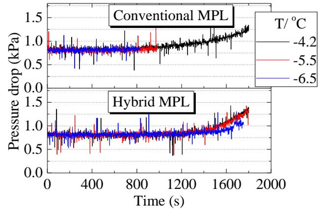
**Fig. 4.** Influence of the MPL on pressure drop in the cathode gas channel at different super-cooling temperatures.
