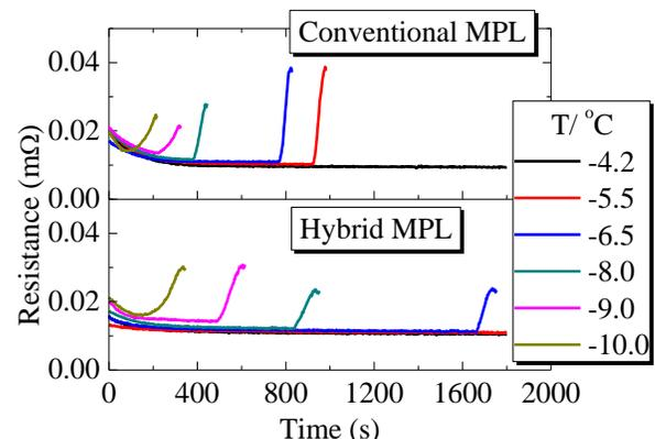
**Fig. 3.** Ohmic resistance changes of PEFCs using conventional and hybrid MPLs when cold starting
