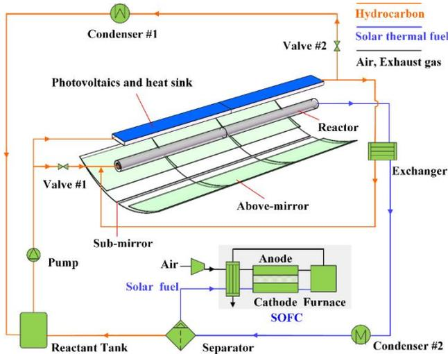
Figure 2. Schematic flow diagram of hybrid prototype
