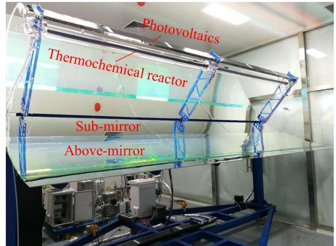
Figure 1. Photo of the prototype of hybrid system
