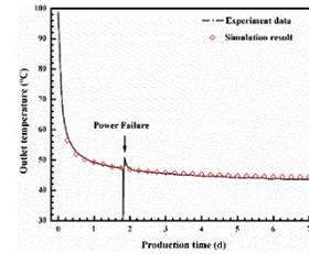
Fig 2 Simulation data and experiment data
