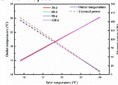
Fig 6 Thermal performance with inlet temperature
