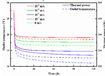
Fig 3 thermal performance with subsurface water velocity
