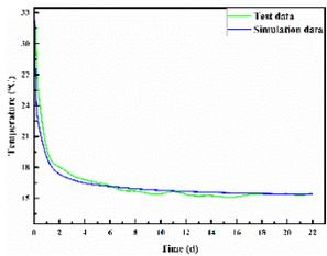
Fig 10 Temperature at 900 m in tubing
