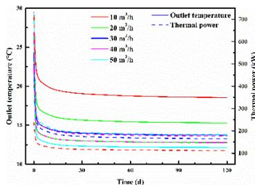
Fig 4 Thermal performance with mass flow
