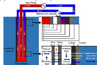
Fig 1 Downhole coaxial heat exchanger
