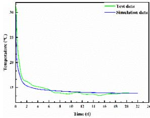
Fig 8 Temperature at 900 m in annulus
