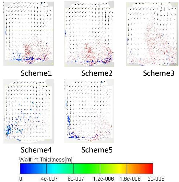
Fig 4 The velocity and wall film thickness distribution in cylinder when inlet closing (549° CA)
