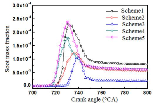
Fig 7 Soot generation process in cylinder
