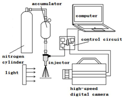
Fig 1 Experimental device of shooting spray
