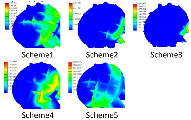
Fig 6 Soot mass fraction distribution in cylinder
