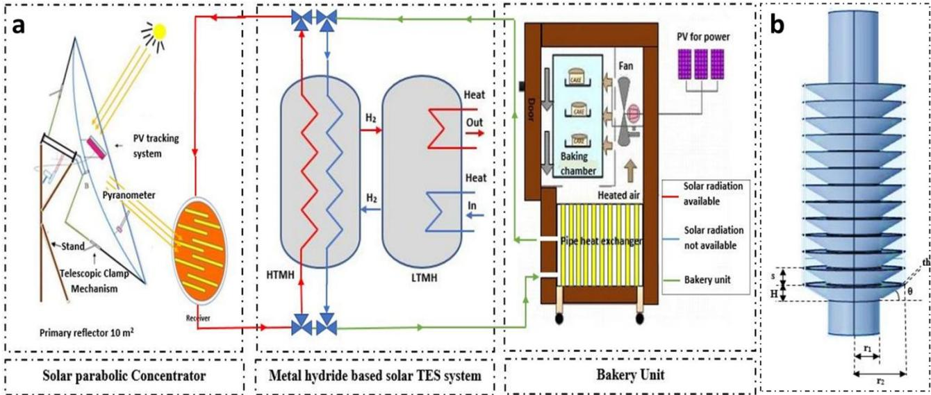
**Fig. 1. a) Schematic diagram of the novel solar bakery unit using MH-TES system b) Design of annular fins type heat exchanger**
