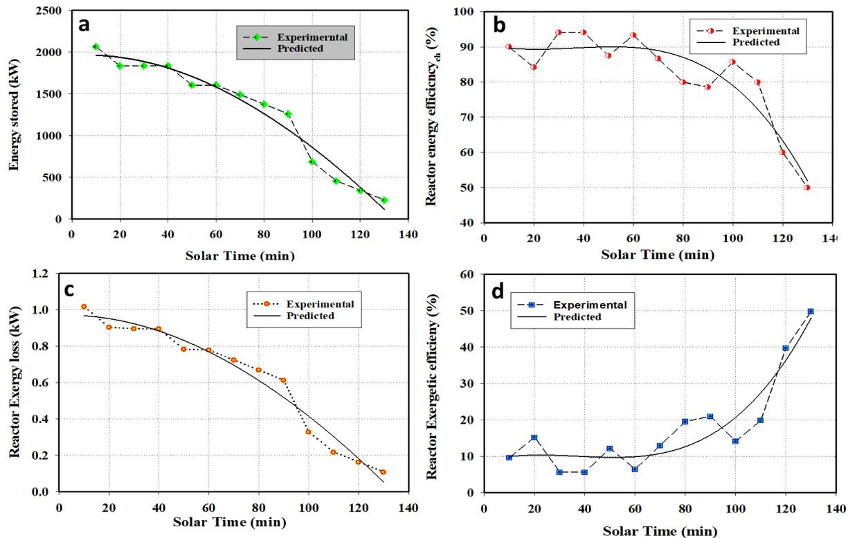
**Fig. 7 Comparative trend between experimental and model predicted parameters: a) rate of energy stored, b) reactor energy efficiency during charging process, c) reactor exergy loss, d) reactor exergy efficiency**
