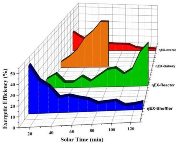
**Fig. 5. Scheme of exergy efficiency of entire system (Scheffler receiver, reactor and bakery unit)**
