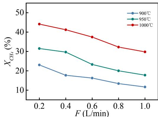
Fig. 4 Methane conversion with different inlet flow rate ( $\text{CH}_4:\text{CO}_2=1$ )
