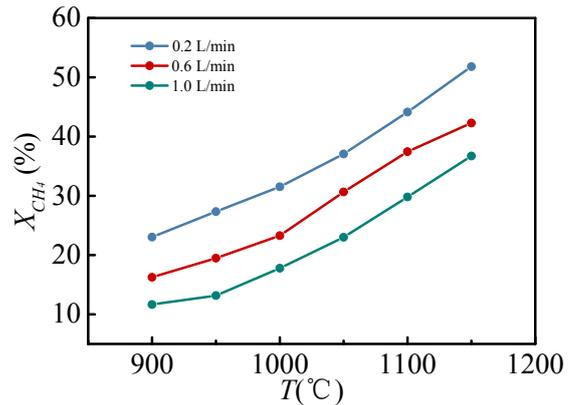
Fig. 3 Methane conversion with different bed temperature ( $\text{CH}_4:\text{CO}_2=1$ )
