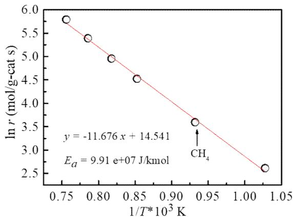
Fig. 5 Arrhenius plot of  $\ln r$  versus  $1/T$  for  $\text{CH}_4$  ( $\text{CH}_4:\text{CO}_2=1$ )
