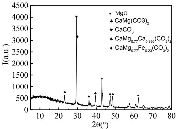
Fig.2 XRD of dolomite decomposition after methane reforming process ( $\text{CH}_4:\text{CO}_2=1$ )
