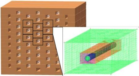
Fig.2 Thermal storage unit structure and mesh generation
