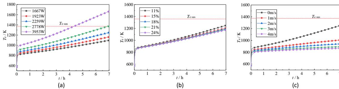
Fig 3 Electric heating wire temperature: (a) different powers (b) different hole ratios (c) different wind speeds
