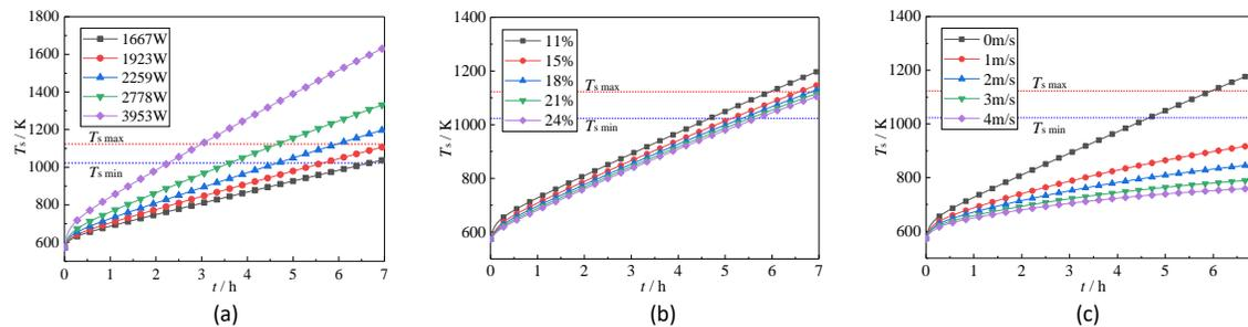
Fig 4 Thermal storage masonry temperature: (a) different powers (b) different hole ratios (c) different wind speeds
