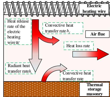
Fig 1 Schematic diagram of heat transfer
