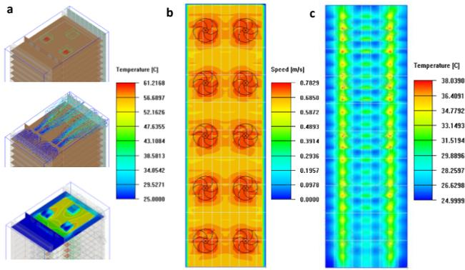
Fig 7 Air side inlet inhomogeneous temperature and wind speed of evaporator under variable heat load conditions
