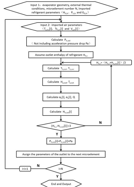
Fig 4 Flow chart of iterative calculation for vertical tube evaporator
