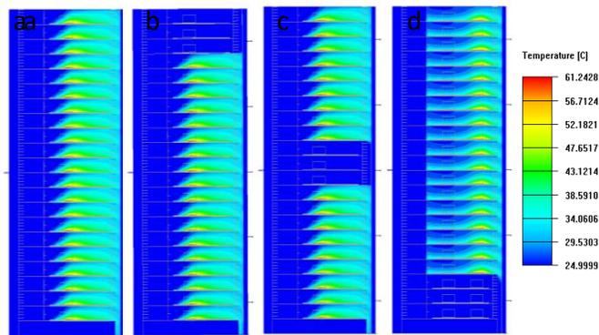
Fig 8 Upper (b), middle (c) and lower (d) parts of the rack are set to zero load
