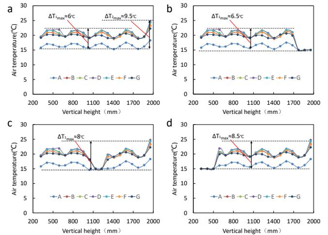
Fig 9 The air side outlet temperature of the evaporator vary with the position of the vertical microelement (a. full load, b. Upper, c. middle, d. lower are set as zero load )
