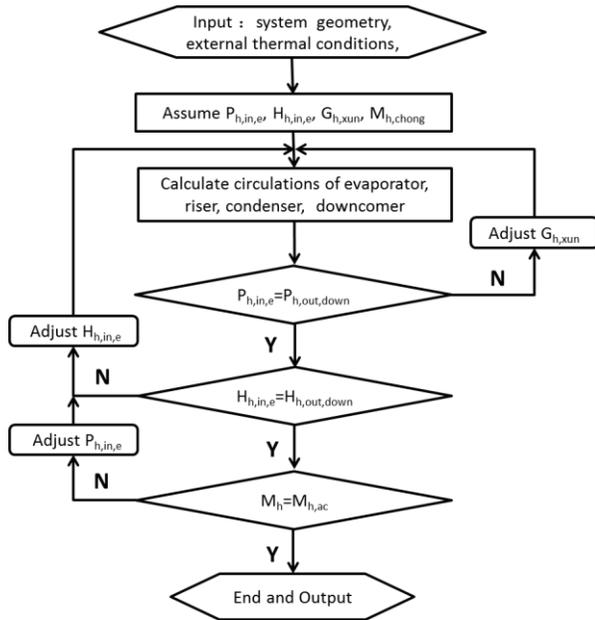
Fig 5 Flow chart of simulation calculation for loop thermosyphon system
