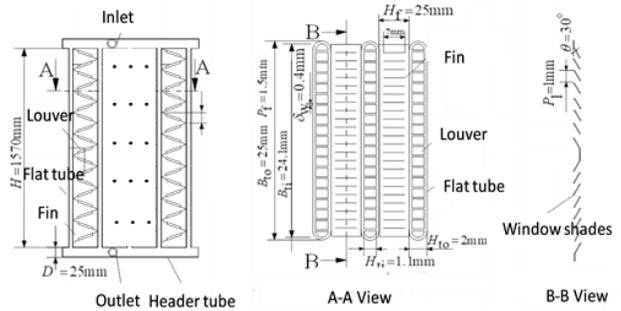
Fig 1 Structure and size of a microchannel flat tube heat exchanger
