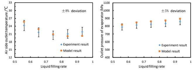
Fig. 6. Comparison between experimental results and model calculation results of air outlet temperature and outlet pressure evaporator
