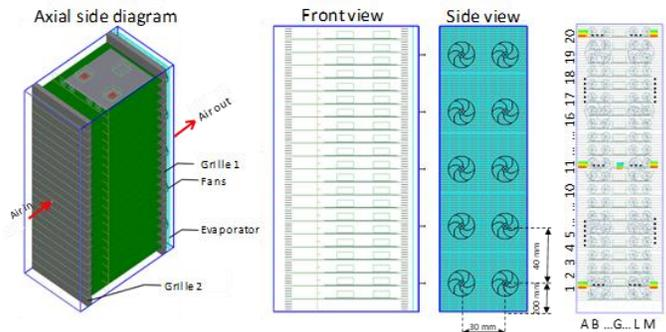
Fig 3 The model structure of the cabinet and the layout of the fans and servers
