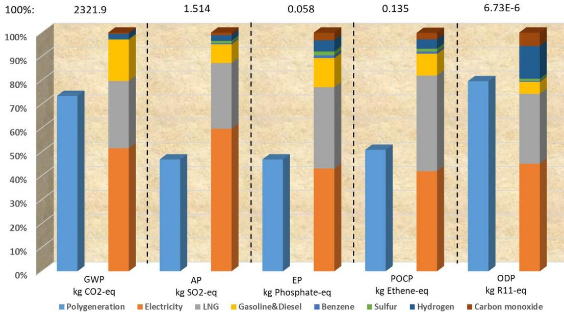
Fig.3. LCA comparison results of the polygeneration system and combination system. The upper values are the absolute life cycle impact category values of combination system, which are esteemed as 100 percent in comparison.
