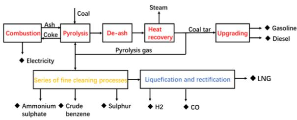
Fig. 1. The schematic technological route diagram of the polygeneration system.
