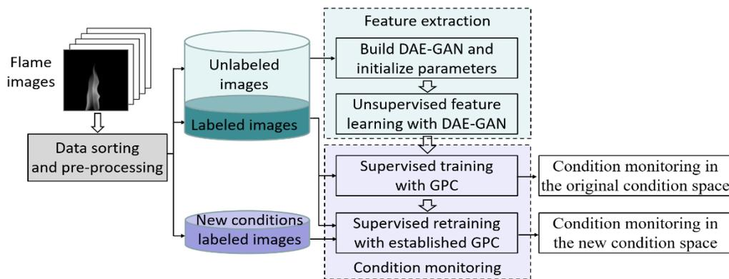
Fig 1 Overall strategy of combustion condition monitoring
