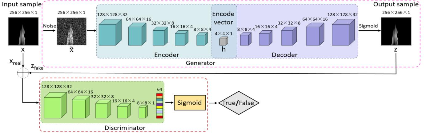
Fig 2 The structure of the designed DAE-GAN
