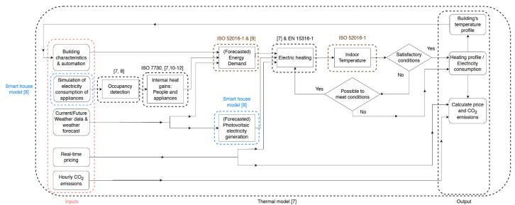
Fig 1 Flow chart describing the model and what is consists of. Blue parts are from the smart house model [8], red parts are inputs to the system, brown parts are calculated according to ISO 52016-1 and [9], electric heating consists of [7] and EN 15316-1, internal heat gain calculations ISO 7730 and [7,10–12] and the rest is according to methods presented in [7].
