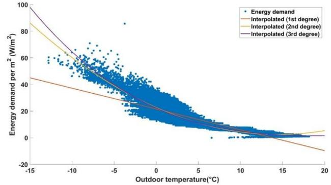
Figure 6. Energy signature curve of DH demand of Cohort 2 under 1<sup>st</sup> degree, 2<sup>nd</sup> degree, and 3<sup>rd</sup> degree polynomial.
