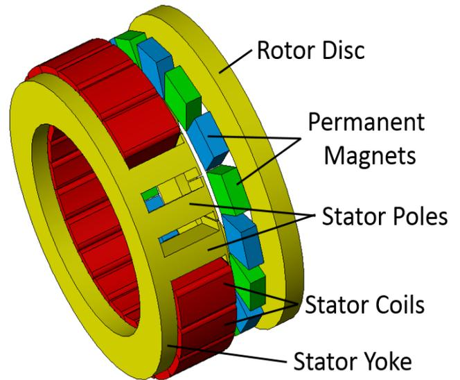
Fig 4 Outline of the axial-flux PMSM topology
