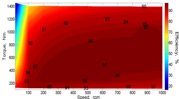
Fig 10 PMSM efficiency map [3]
