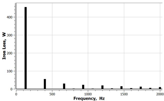
Fig 6 Stator iron losses
