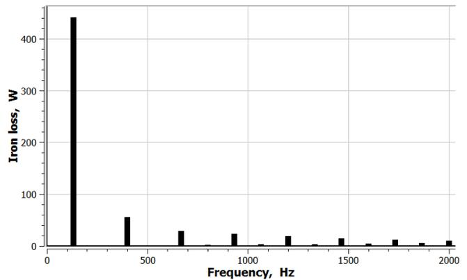
Fig 8 Stator iron losses
