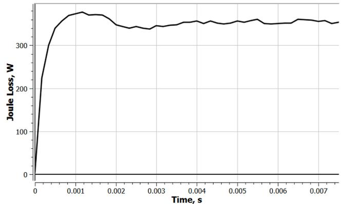
Fig 7 Rotor eddy currents Joule losses plus stator windings Joule losses
