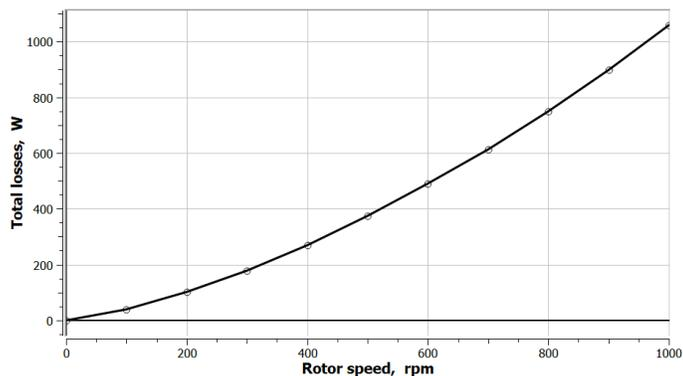
Fig 9 No-load losses for the entire rotor speed range
