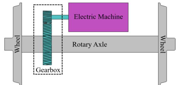
Fig 1 Drive system with transmission
