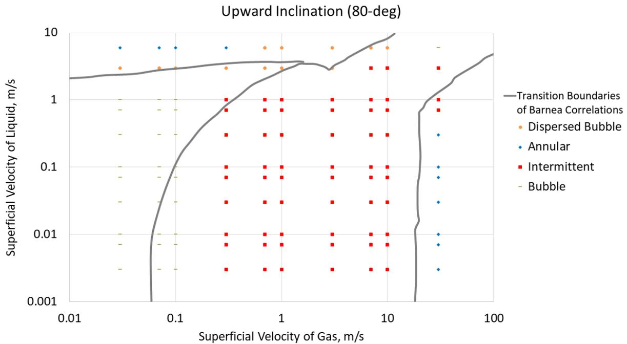
**Fig 5** Comparison of flow pattern predictions between ANN model (dotted points) and Barnea correlations (full lines) during air-water two-phase flow in a 2-inch, upward inclined (80°) pipe at atmospheric conditions. water (0.003 ~ 6 m/s), and inclination angles (0°, 1°, 30°, 80°, and 90°).
