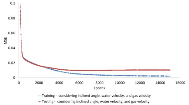
**Fig 3** Variations of mean squared error (MSE) over 15000 iterations of the ANN training and testing loops.
