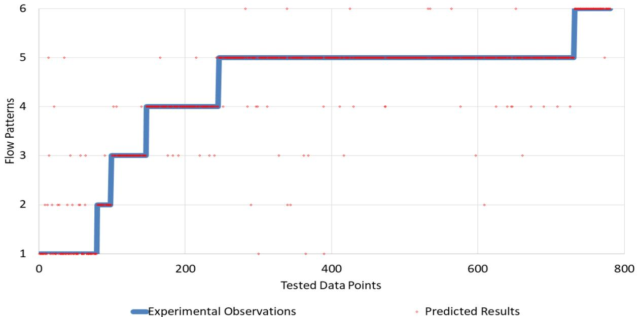
**Fig 4** Comparisons of experimental and predicted flow patterns during air-water two-phase flow in a 2-inch pipe at atmospheric conditions and different inclined angles.
