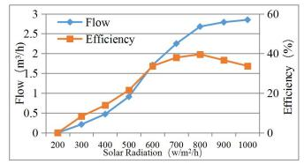
Fig 4 Characteristic of 3 kW solar water pumping system
