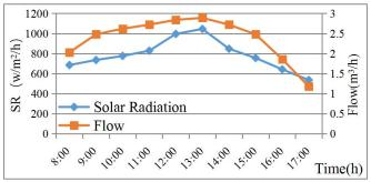
Fig 2 Diurnal variation of solar radiation and water flow in July
