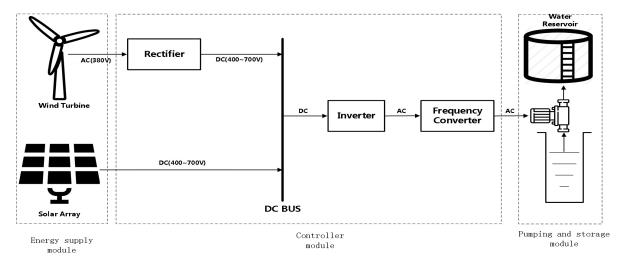
Fig 1 Schematic diagram of wind-solar complementary water supply technology
