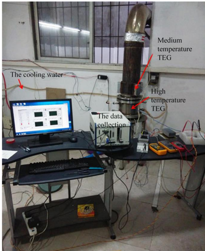
Fig.4 Experimental facility of the high-temperature and medium-temperature coupled TEG system
