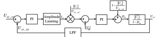
Fig.6 The control scheme of the ACTIVE PFC
