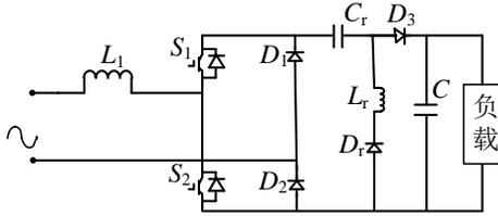
Fig.1 The basic structure of the ACTIVE PFC
