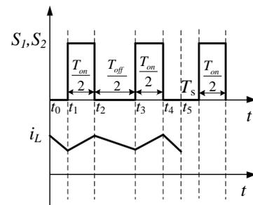
Fig.4 the working mode of the double peak PWM
