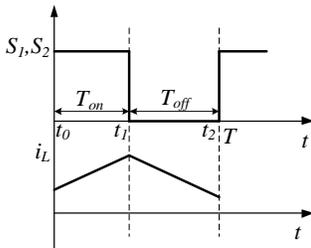
Fig.2 Two working mode of the single PWM
