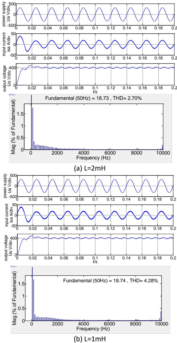
Fig.7 The waveforms of power supply  $U_a$ , input current  $i_{sa}$ , and output voltage  $U_o$ , and  $i_{sa}$  THD with the single PWM
