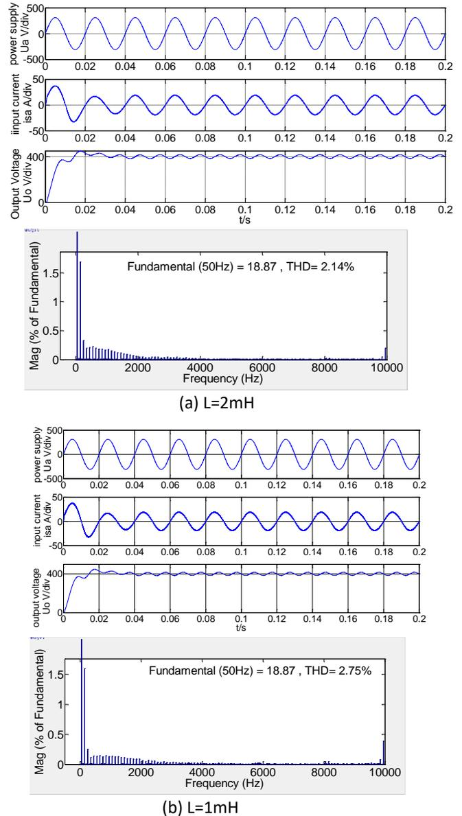
Fig.8 The waveforms of power supply  $U_a$ , input current  $i_{sa}$ , and output voltage  $U_o$ , and  $i_{sa}$  THD with the double peak PWM
