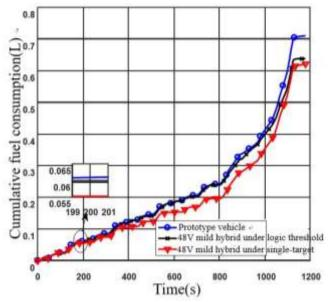
Fig 8. Comparison of cumulative fuel consumption
