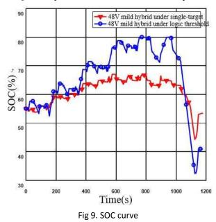
It can be seen from the figure 9 that the initial SOC values of both are 55%. After a NEDC operating cycle, the battery SOC of the 48V mild hybrid vehicle under the
