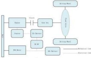
Fig 1. 48V system structure
