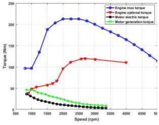
Fig 3. Engine and motor characteristic curves
