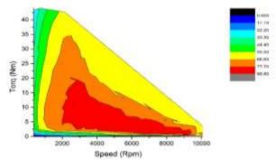
Fig 2. Efficiency MAP diagram of the motor
