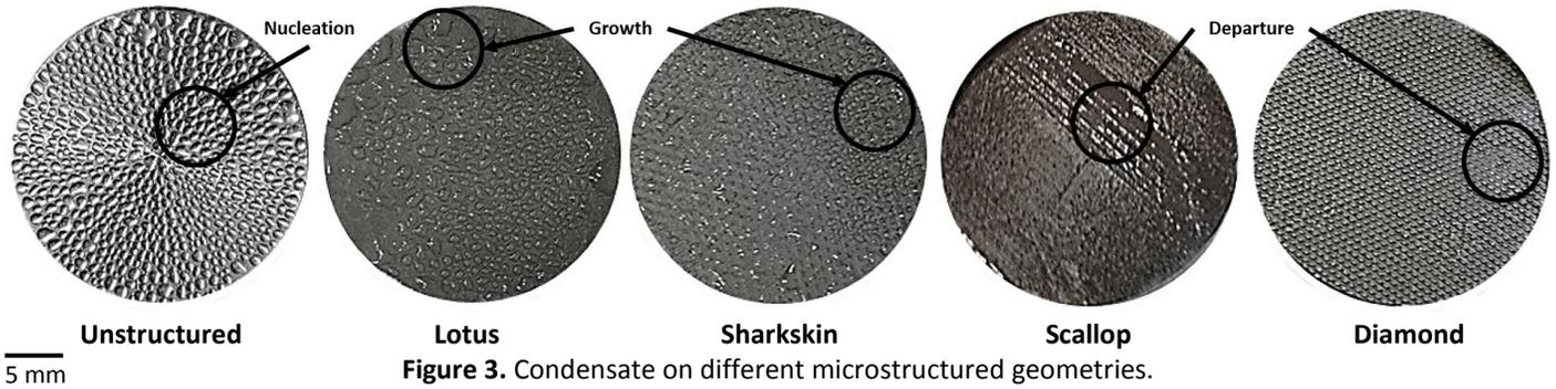
Figure 3. Condensate on different microstructured geometries.
