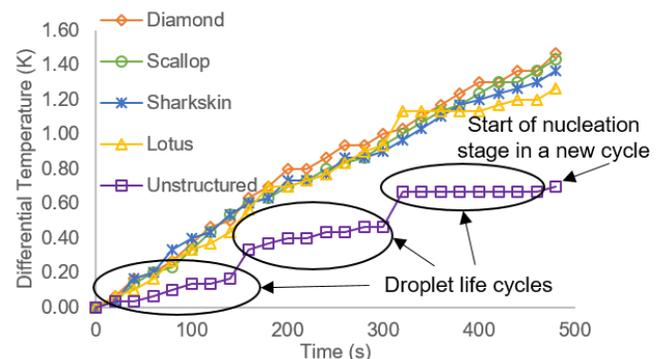
Figure 4. Differential Temperature ( $\Delta T$ ) vs. Time.
