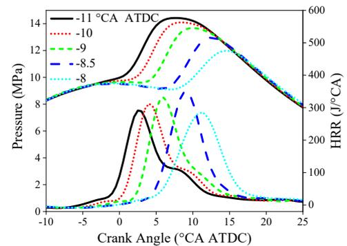
(a) In-cylinder pressure and heat release rate
