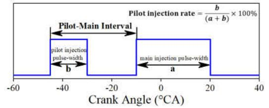
Figure 2. Definition of the pilot injection rate
