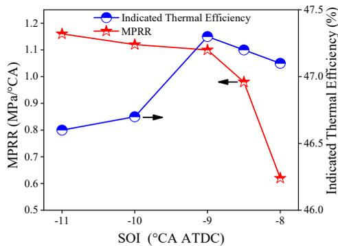
**Figure 4.** The MPRR and indicated thermal efficiency at different SOI
