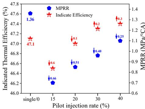
**Figure 8.** The indicated thermal efficiency and MPRR of different injection strategies
