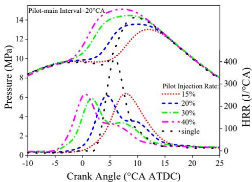
(b) The effect of different pilot injection rates with a 20 °CA interval
