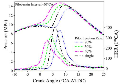
(c) The effect of different pilot injection rates with a 50 °CA interval
