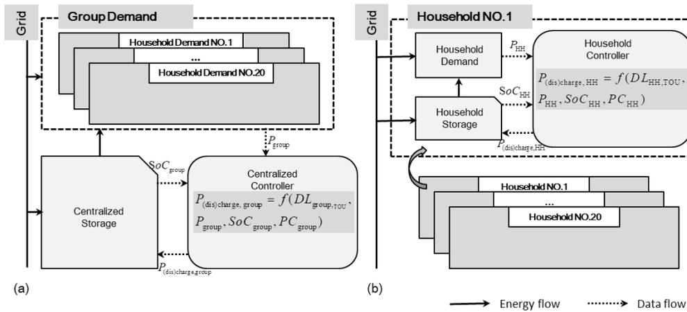
Fig. 1. Storage configurations: (a) Centralized storage and (b) distributed storage configurations
