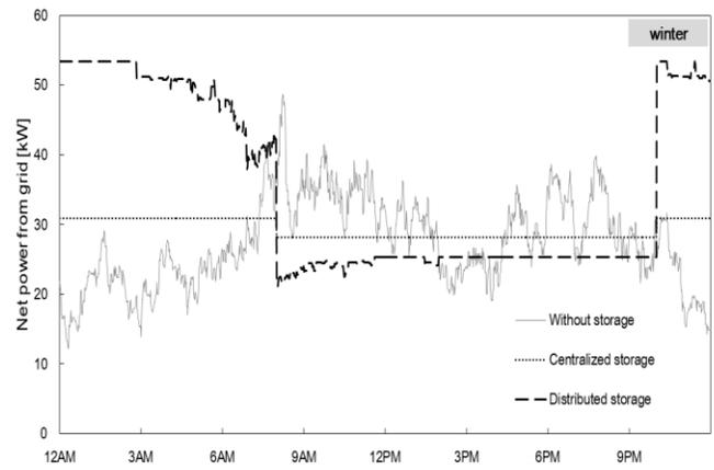
Fig 3 Net power from grid of 20 households without storage, with centralized and distributed storage
