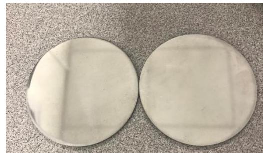
Fig.2. Image of slab samples used for thermal conductivity test
