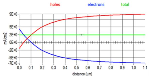
Fig 6 Current density of the optimized Cu<sub>2</sub>O/TiO<sub>2</sub> heterojunction solar cells.
