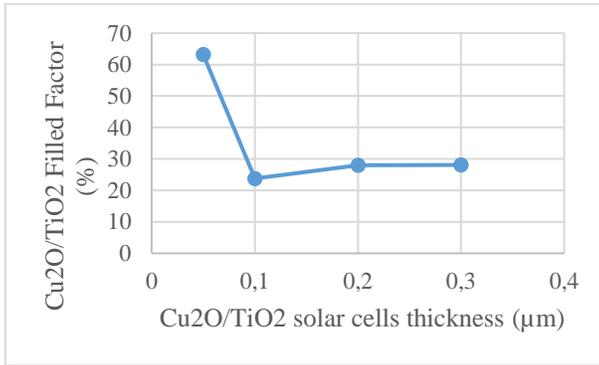
Fig 3 A plot of absorber and buffer layer thickness with the solar cells filled factor.
