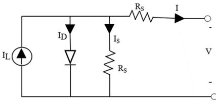
Fig 1 Solar cells model equivalent circuit
