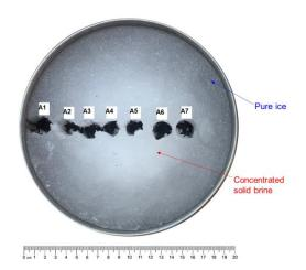
Fig 4 Radially frozen salt-water solution (Sol. A) and samples locations, total volume ~1570mL frozen at -20°C for 24 hours
