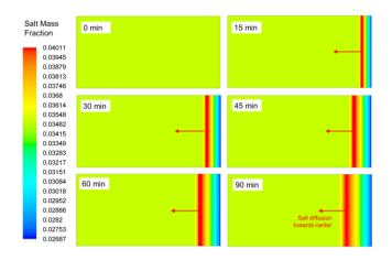
Fig 8 Contours of salt mass fraction showing the salt diffusion towards the center of the crystallizer running at freezing temperature of -20°C
