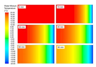
Fig 6 Temperature contours of water mixture in a crystallizer with radial directional freezing at a temperature of -20C°
