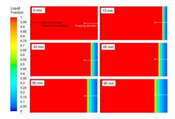
Fig 7 Contours of liquid fraction varying from 0 to 1 captured at the symmetrical section of the crystallizers showing the radial directional freezing at different flow time
