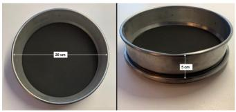
Fig 1 Cylindrical apparatus serves as the crystallizer for directional freezing experiment
