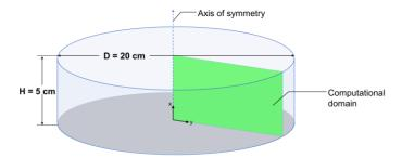
Fig 2 Geometry of the crystallizer and the axisymmetric modelling domain
