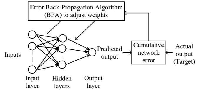
Fig 2 A schematic diagram for multi-layer feed-forward ANN model with an error back-propagation training algorithm
