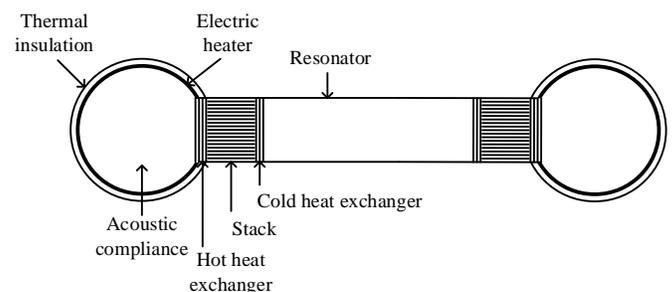
Fig 1 Schematic diagram for twin standing-wave thermoacoustic heat engine
