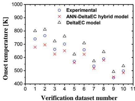
Fig 7 Experimental and predicted onset temperature by both DeltaEC and hybrid models vs. verification dataset numbers
