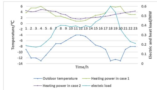
Fig 5 Outdoor temperature and electric heat load curve
