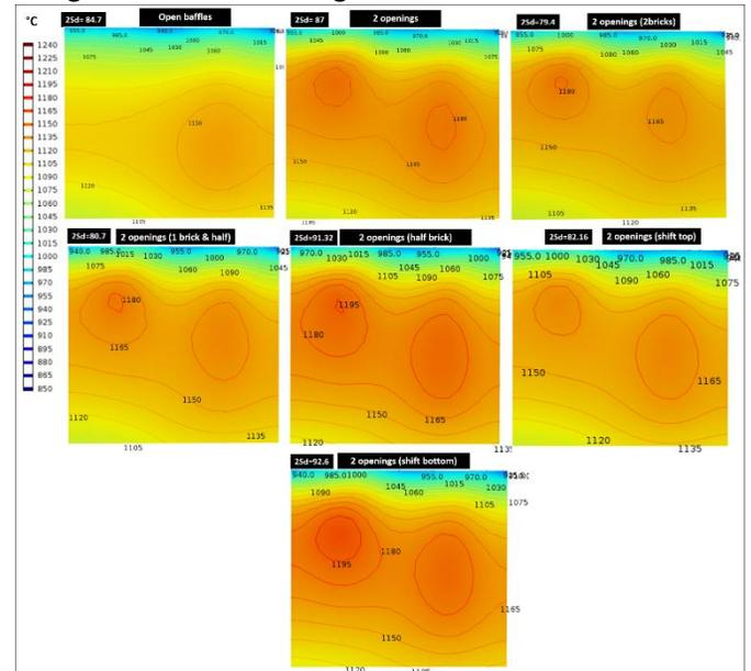
Fig 5 Anode map temperature at the mid-plane for a damaged flue wall for different designs
