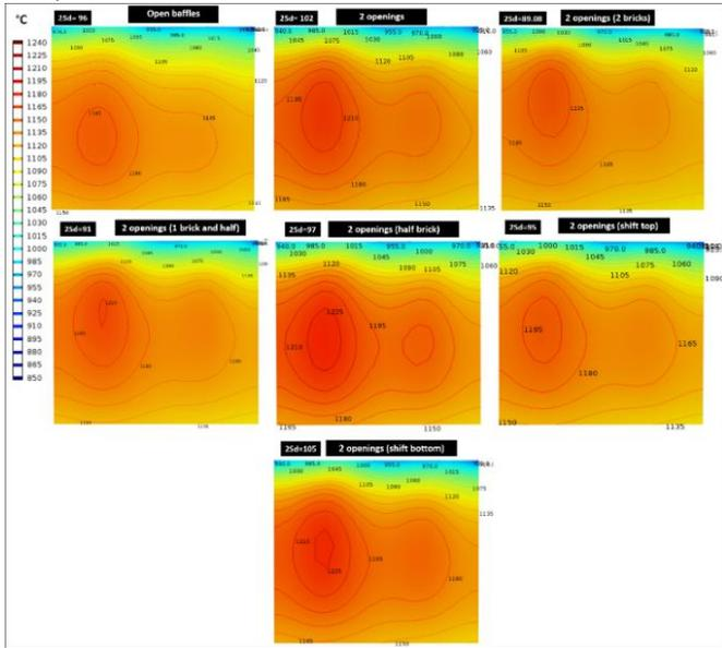
Fig 3 Anode temperature at the mid-plane for new flue wall for different designs
