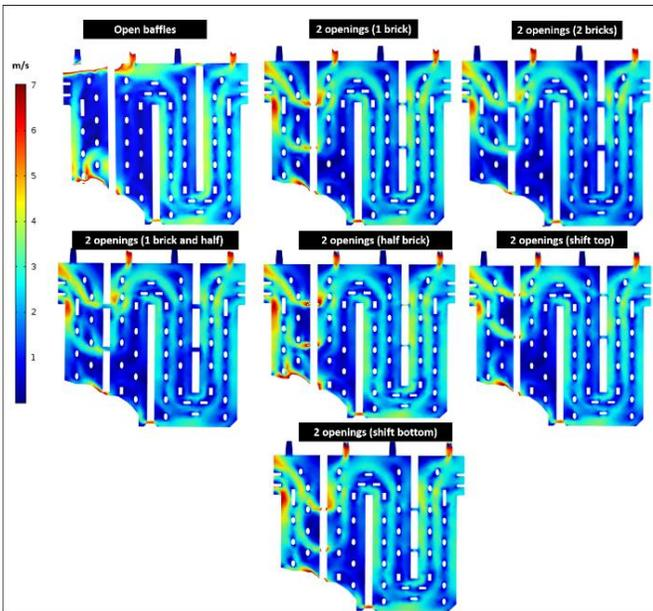
Fig 4 Velocity contours for flow-blockage in different flue-wall designs
