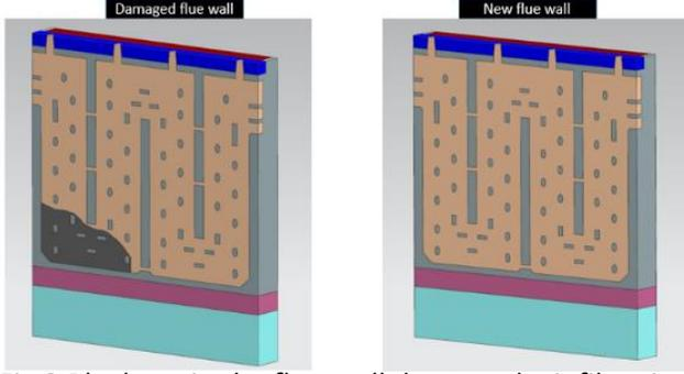
Fig 2 Blockage in the flue-wall due to coke infiltration
