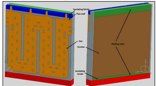
Fig 1 solid and gas computational domains, coupled at the interface
