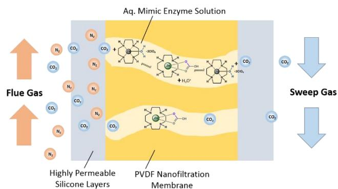
Fig. 1 Schematic of the composite supported liquid membrane separating CO<sub>2</sub>.
