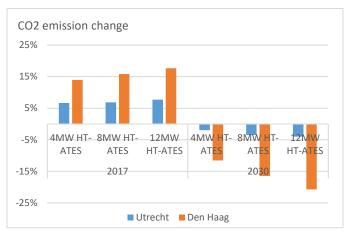
Fig 2.  $\mbox{CO}_2$  emission changes comparing to the sceanrios without HT-ATES
