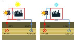
Fig. 1. Schematic diagram of a simple two-well HT-ATES
