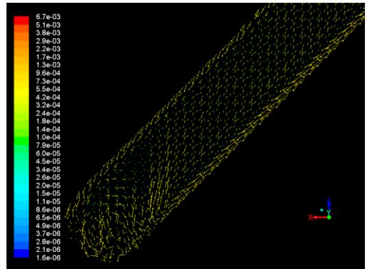
c<sub>2</sub>. Velocity vector map at the bottom of vacuum tube after cooling for 2 h
