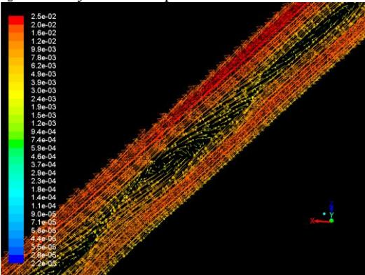
b<sub>1</sub>. Velocity vector map in the middle of vacuum tube in initial state
