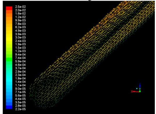
c<sub>1</sub>. Velocity vector map at the bottom of vacuum tube in initial state
