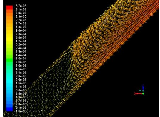
b<sub>2</sub>. Velocity vector map in the middle of vacuum tube after cooling for 2 h
