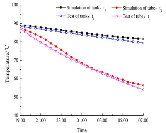
Fig.4 Comparison of the temperature of water heater by simulation and test
