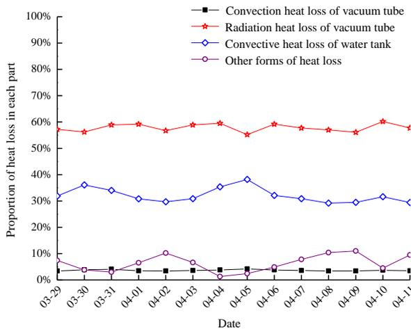
Figure 3 The proportion of heat loss of each part of solar water heater to the actual total heat loss
