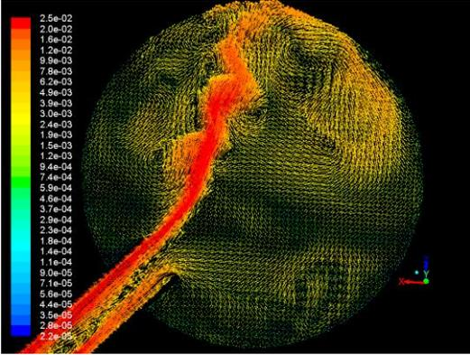
a<sub>1</sub>. Velocity vector map in water tank in initial state
