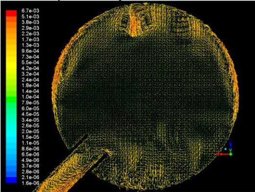
a<sub>2</sub>. Velocity vector map in water tank after cooling for 2 h
