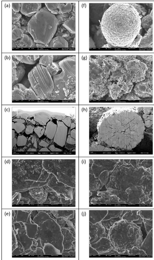
Fig 2 SEM images of (a) fresh single crystal cathode, (b) aging single crystal cathode, (c) cross-section of aging crystal cathode, (d) fresh anode of single crystal anode, (e) fresh anode of poly crystal anode, (f) fresh poly crystal cathode, (g) aging poly crystal cathode, (h) cross-section of aging poly cathode, (i) aging anode of single crystal anode, (j) aging anode of poly crystal anode,
