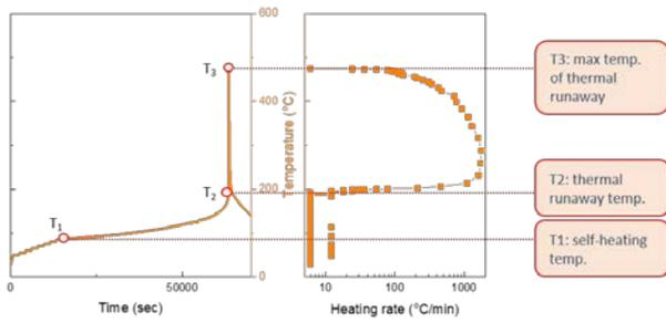
Fig 1 Introduction of thermal runaway and the important parameters  $T_1$ ,  $T_2$  and  $T_3$
