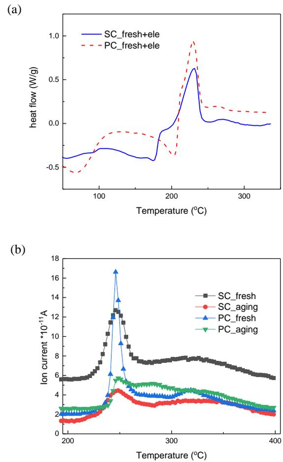
Fig 4 (a) The DSC result of the different cathode with electrolyte adding (b) the  $O_2$  ion current from MS detection
