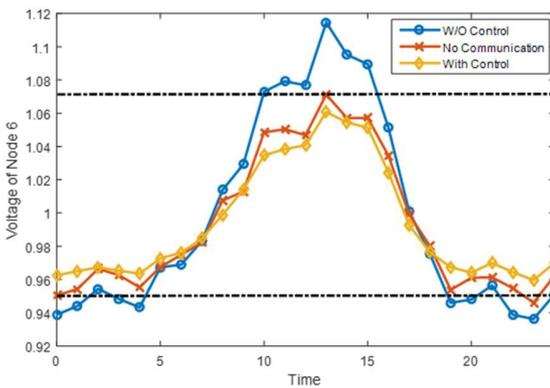
Fig 4 Voltage variation curve of bus 6 in 33 buses system in 24 hours
