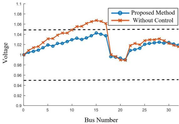
Fig 3 Voltage profiles under the proposed control method and no control
