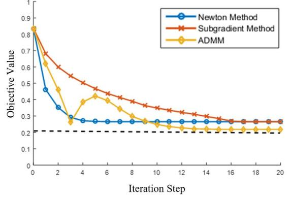
Fig 2 Convergence speed comparison of three methods in 33 buses system
