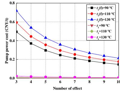
Fig. 7 The pump power cost in terms of MED stage under different first stage temperatures
