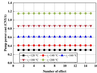
Fig. 8 The pump power cost in terms of number of stage
