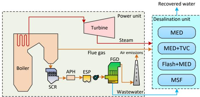
Fig. 1 Schematic of FGD wastewater recovery schemes
