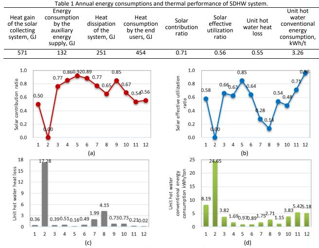
Fig 4 Monthly thermal performance indicator of SDHW system.
