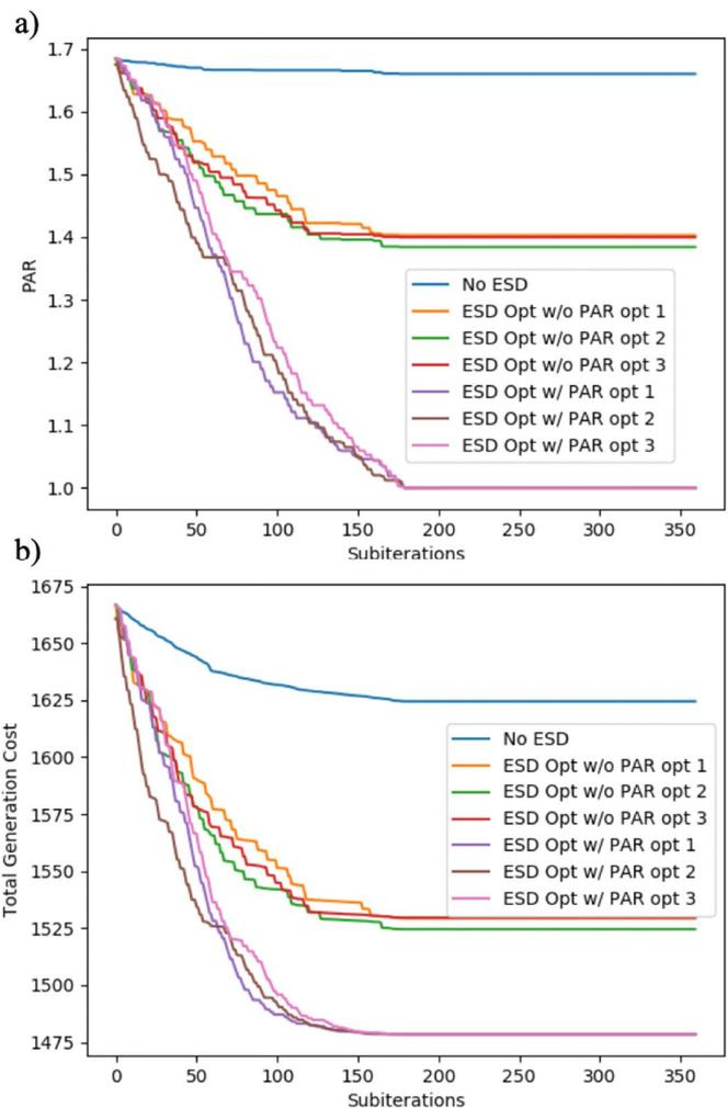
Fig 3 PAR and total generation cost. a) PAR for every iteration for a total of 360 iterations with base opt and 6 ESD opt runs. b) Total generation cost for every interaction for a total of 360 iterations with base opt and 6 ESD opt runs.
