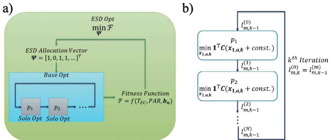
Fig 1 Optimization model. a) The three levels of optimization in the model. b) Depiction of the base opt procedure.
