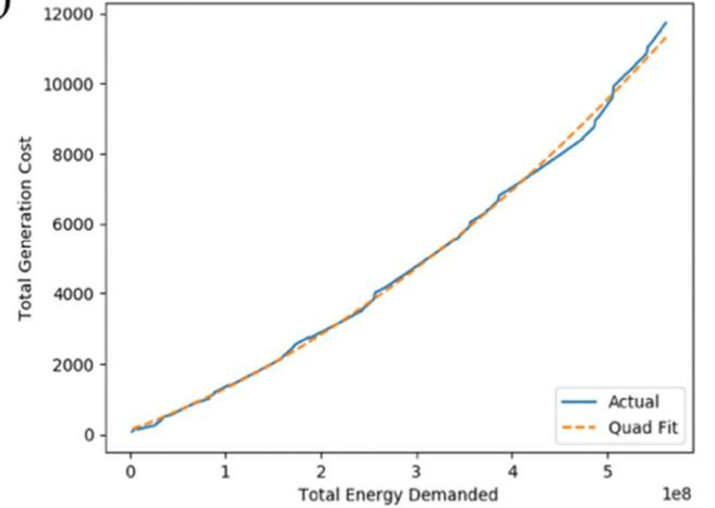
Fig 2 Cost function of CTG. a) MICP model for solving optimal  $C_T$ . b) Regressed CTG quadratic cost function.
