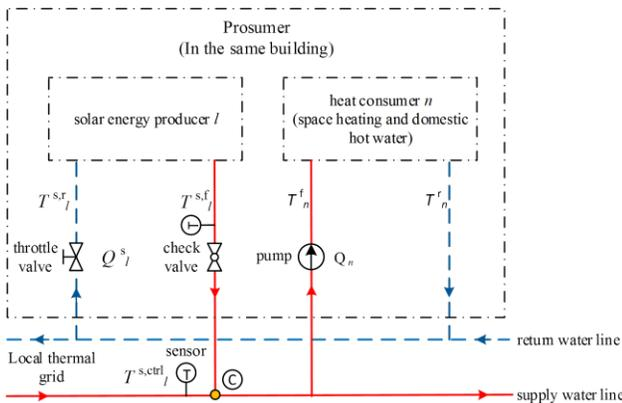
Fig.2.1 Hydraulic connection of a prosumer
