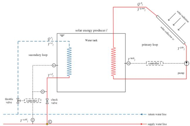
Fig.2.2 Configuration of a solar energy producer /
