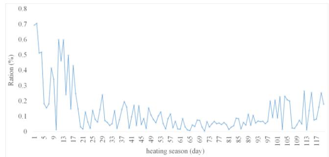
Fig. 5 the ratio between the utilized solar heat and the total supplied heat
