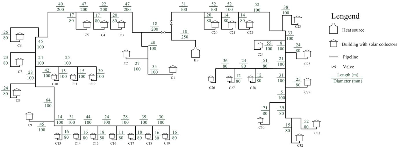
Fig.3 A DH system with solar heating prosumers.
