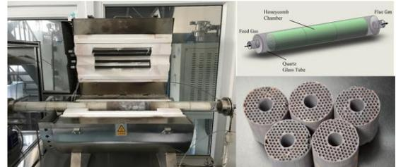
Figure 2 The configuration diagram for the honeycomb reactor and the honeycomb oxygen carrier.
