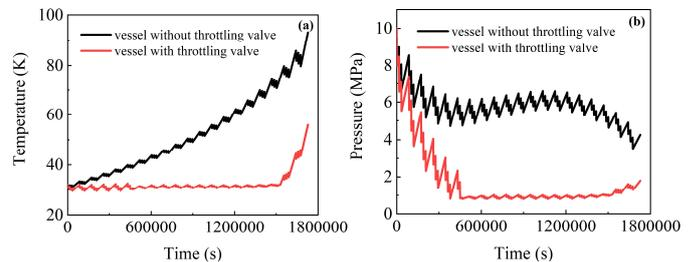
Fig. 7 Changes of temperature (a), pressure (b) for middle-initial-pressure vessels.
