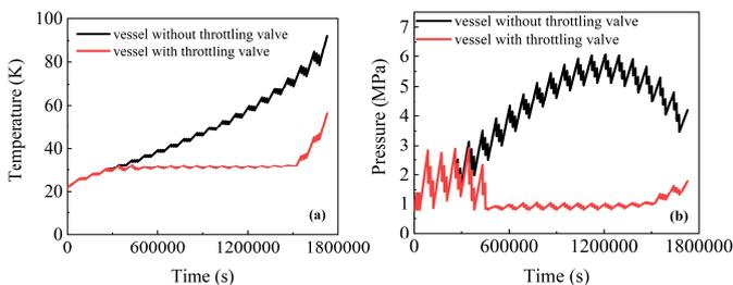
Fig. 6-Changes of temperature (a), pressure (b) for low-initial-
