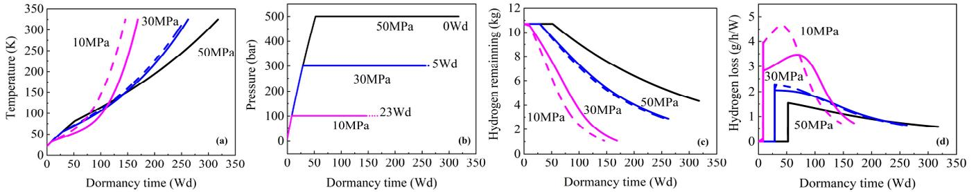
Fig. 4-Comparison of temperature (a), pressure (b), hydrogen remaining (c), hydrogen loss rate (d) between the vessel with a throttling valve and vessel without throttling valve. The solid lines denote the results for the vessel with a throttling valve, while the dashed lines denote the results for the vessel without throttling valve. Initial conditions:  $m_{H_2}=10.7$  kg,  $P=1$  MPa,  $T=21.4$  K.
