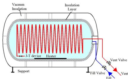
Fig. 1- The schematic diagram of hydrogen vessels with a throttling valve
