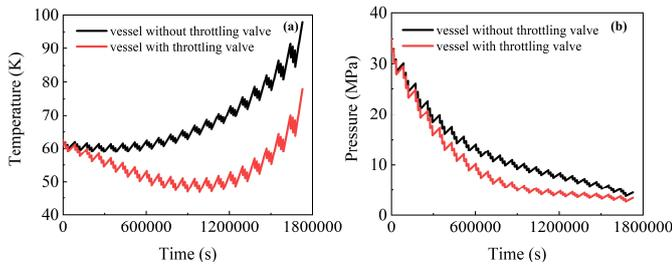
Fig. 8 Changes of temperature (a), pressure (b) for high-initial-pressure vessels
