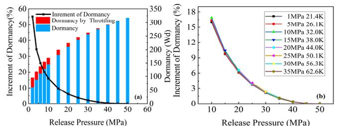
Fig. 3-Increment of dormancy with a throttling valve in the vessels at different release pressures (a), initial pressures (b).
