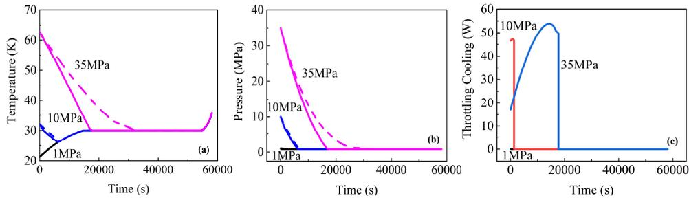
Fig. 5- Change in the thermodynamic state of hydrogen in the process of discharge. (a)temperature, (b)pressure, (c)throttling cooling capacity. The solid lines denote the results for vessels with a throttling valve, while the dashed lines denote the results for vessels without throttling valve.
