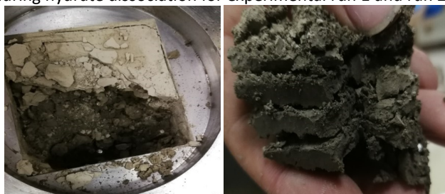
Fig. 7 Inner structure of sea muds after hydrate dissociation for Run2.
