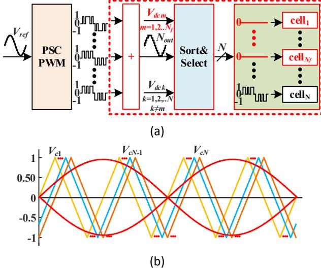
Fig. 4. Proposed PS PWM and sort&select algorithm under grid fault condition. (a) Overall diagram of the modulation process. (b) Principle of PS PWM.
