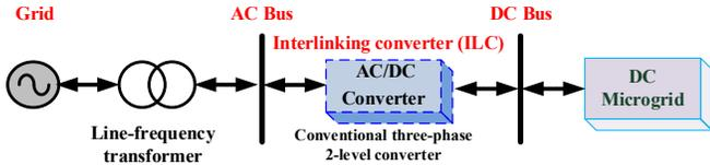
Fig. 1. Conventional low-voltage hybrid AC/DC microgrid.
