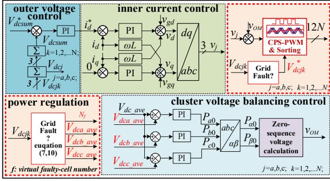
Fig. 3. The overall controller with grid fault-tolerant ability.
