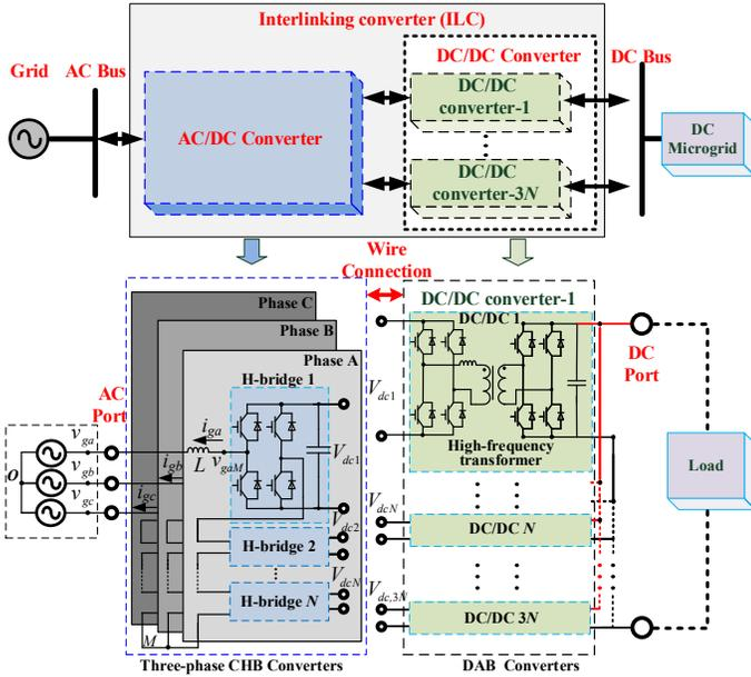
Fig. 2. The proposed MV hybrid AC/DC microgrid.
