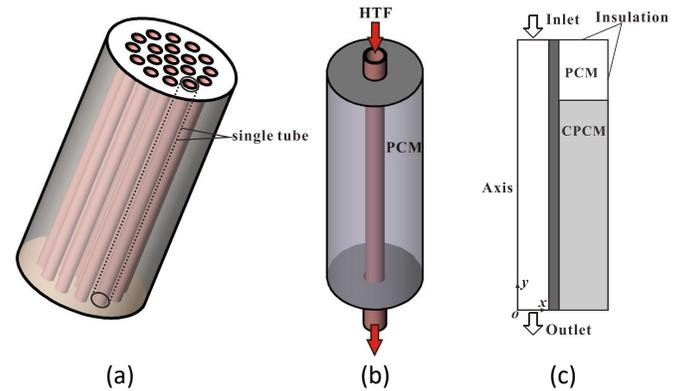
Fig 1 (a) Thermal energy storage tank; (b) Physical model; (c) Computational domain
