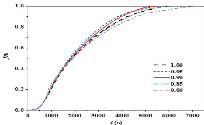
Fig 3 Melting fraction as a function of time for different filling ratios
